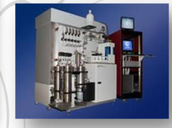
Core Flood System
